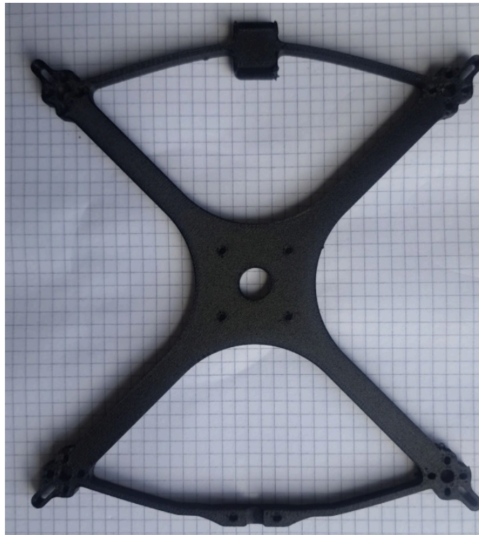
Figure 35: The custom 3D-printed Quadcopter Frame
