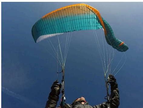
Figure 1: Asymmetrical Canopy Collapse [1]
