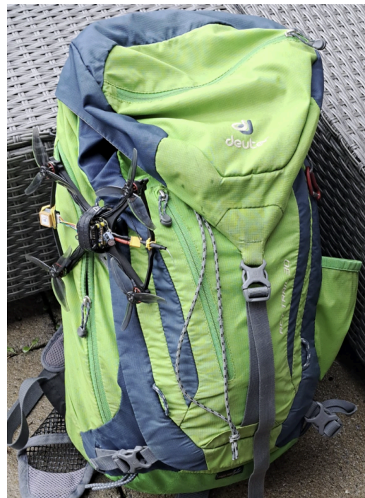
Figure 57: The Quadcopter clipped onto a standard Hiking Backpack using the Battery Latch
