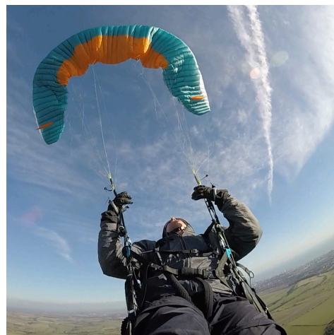
Figure 2: Frontal Canopy Collapse [1]
