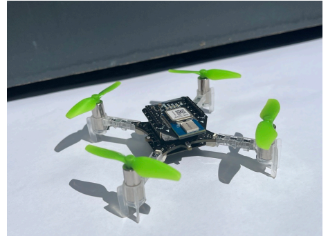
Figure 7: Crazyflie 2.1 equipped with a Flow Deck v2 and a Loco Positioning Deck.
