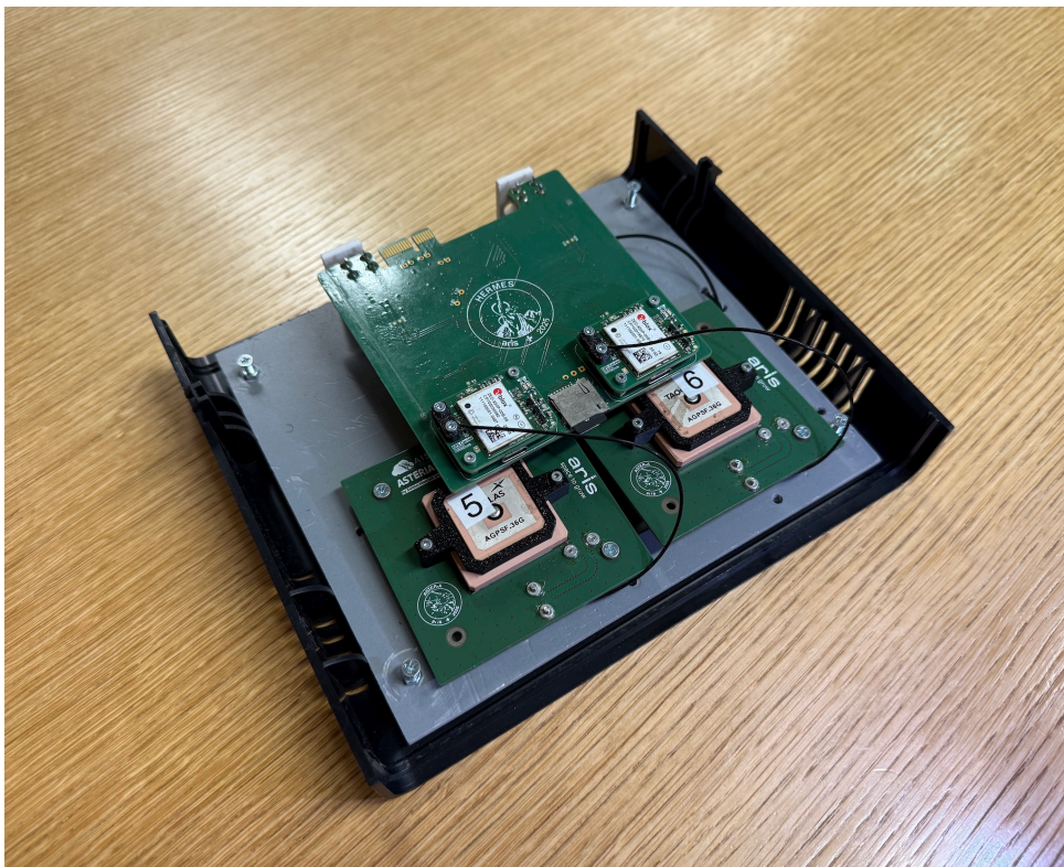
Figure 59: Housing used to hold the ASTERIA boards in place during the car drives.
