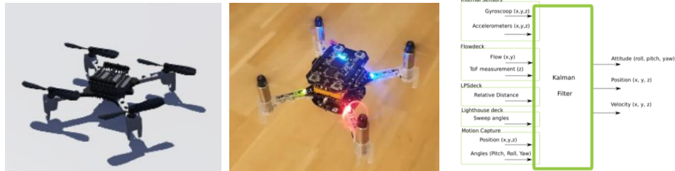
Figure 2: A Crazyflie 2.1 miniature quadcopter in simulation 5,6 (left) and real flight (center) performs state estimation with an EKF model 7 (right) for a fully instrumented Crazyflie platform.
