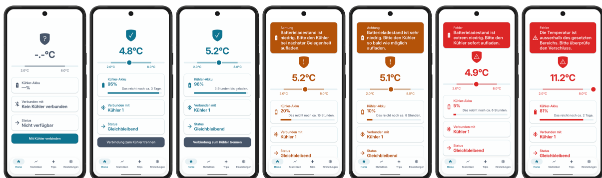
Figure 28: Home screen in different states: disconnected, connected with charging and discharging battery, battery warnings, battery errors and temperature errors.
