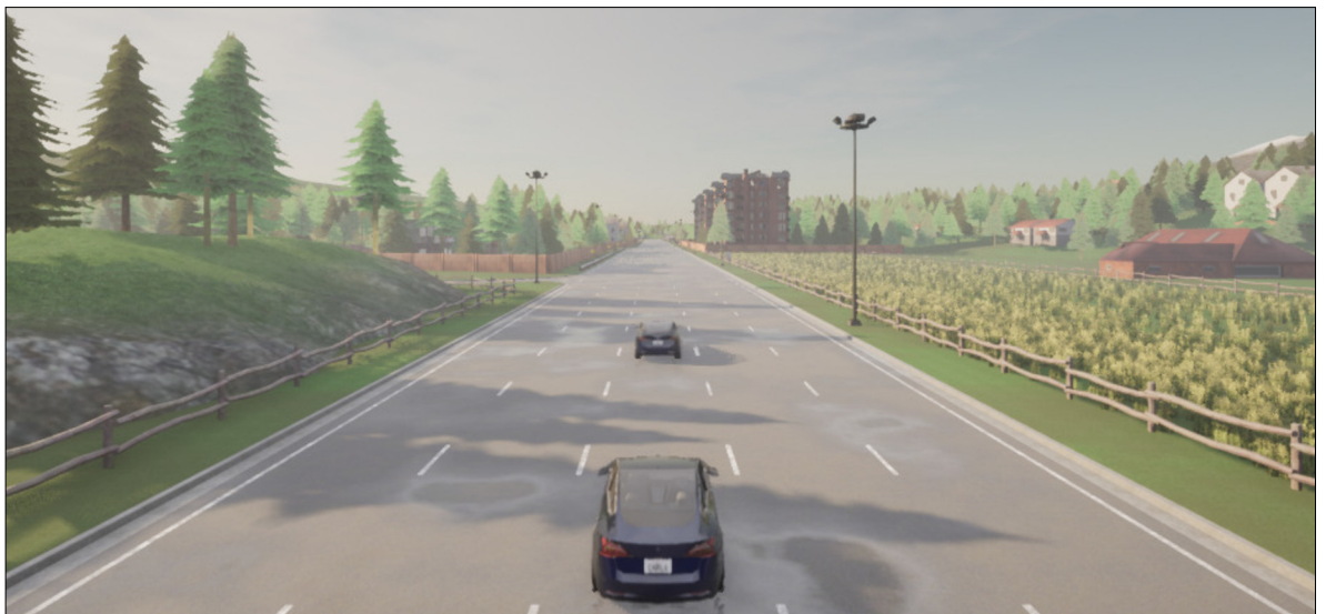
Vehicle platooning situation in the CARLA simulator with the leader and follower car. Own presentation
