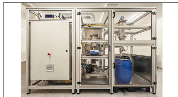
Fig. 3: Left side of the prototype. Centre: Crystallisation Vessel. Right: Sedimentation Vessel. Left: Control cabinet Own presentation
