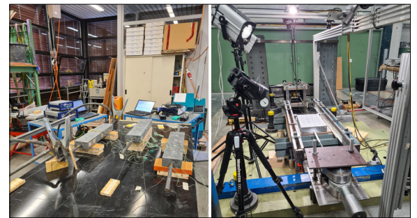
Fig. 1: Test setup of the activation tests and pull-out tests with long embedment length Own presentation
