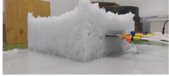
Figure 10: Wet snow block prepared with the first method. The block has many air gaps, and a distinctly wetter layer is visible at the bottom.
