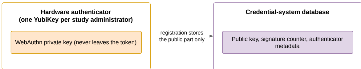
Figure 8.12.: Storage of the operator-authentication keys.
