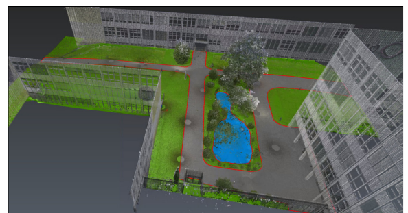
Mesh extraction of the Buchs campus in Leica Cyclone 3DR Own presentation
