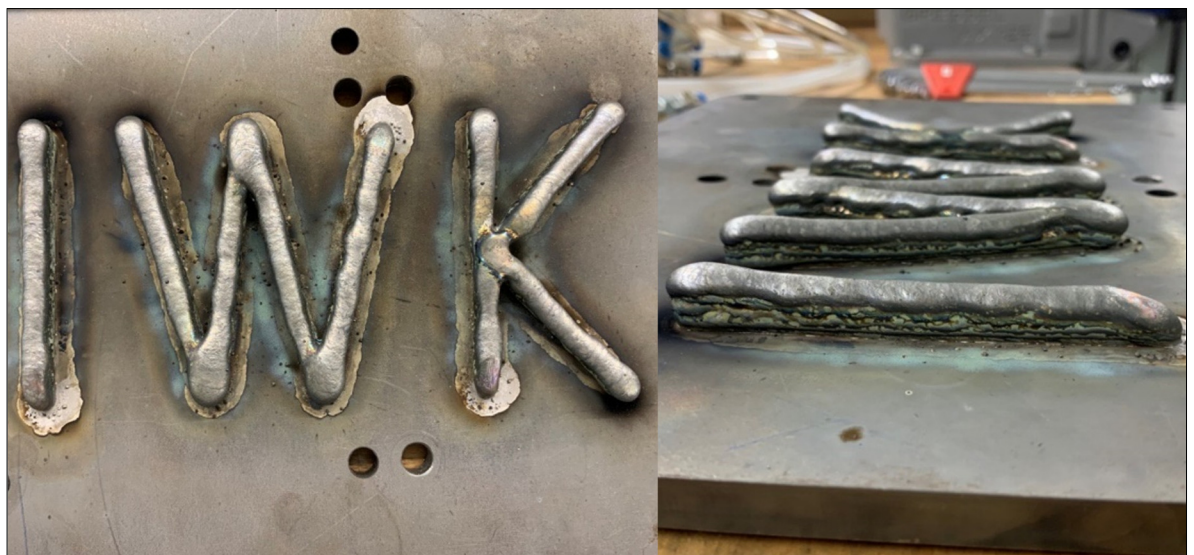
side and top view of demonstrator, NiCr22Mo9Nb deposited onto DC04 mild steel plate Own presentation
