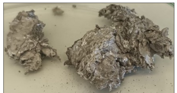
Image of liquid metal after reaction with carbon dioxide in bubble column reactor to form gallium oxide and solid carbon Own presentment
