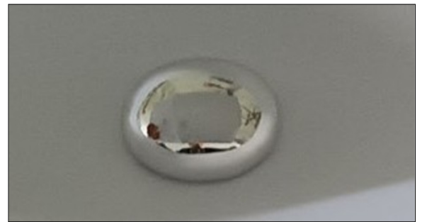
Droplet of the liquid metal used in project for carbon capture: the eutectic alloy of gallium, indium and tin Own presentment
